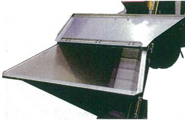
Heating. The feeding hopper, equipped with cover and heater, keeps the garlic temperature before the peeling process.
