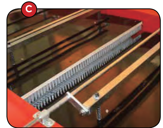
C. Two top brushing sheets with double regulation adjust the brushing strength.
