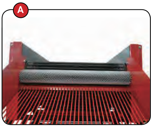
A. A three working methods combined among the riveted rod belt, brush and the bars grill separate the clods and soil from the bulbs.
