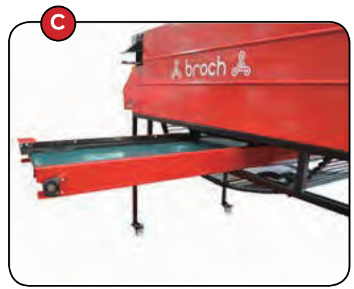
C. The clods, soil, and removed rests are collected and unloaded through the rubber belt to the trash boxes.
