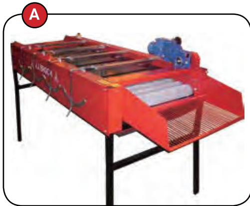
A. 3m brushing up and down remove efficiently the soil and the external brown peels.
