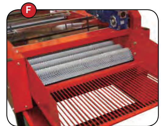
F. The final screen separates the rest of soil and avoids getting it into container.
