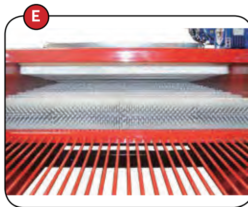
E. The specific synthetic filaments brushes provide excellent rotation to ensure thorough cleaning of garlic bulbs.
