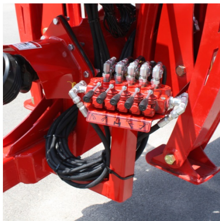
Hydraulic Spool Valve Control
