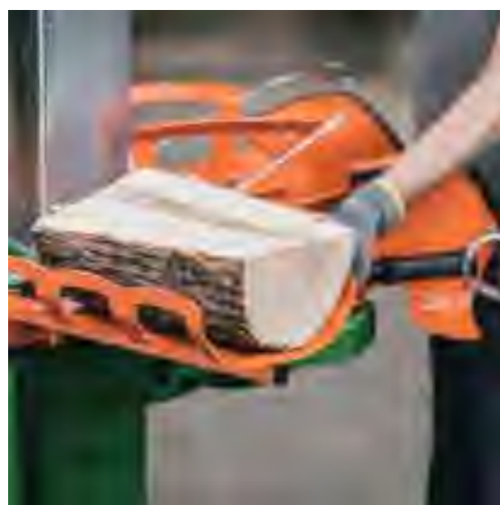
Wood pieces to be split, but also already split logs can be comfortably placed on the wood shelves on both sides of the machine.
