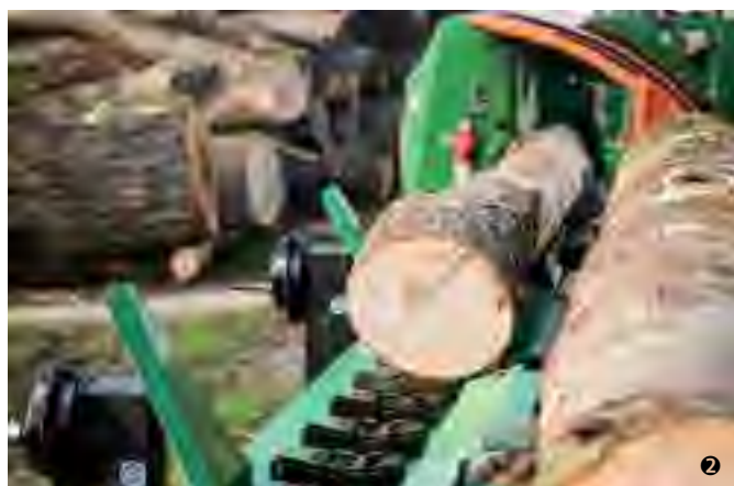
Constant supply of the log feeding system consisting of 1 cross conveyor and 2 longitudinal conveyor.
